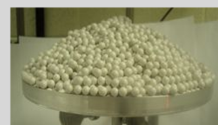
Figure 3: Pellet pile that acts as our sand pile on the base plate.
